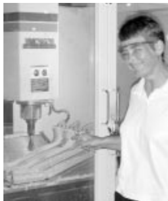
Lori Rydberg, Director of Operations at Gibson, points out a CNC carver shaping intricate guitar necks
