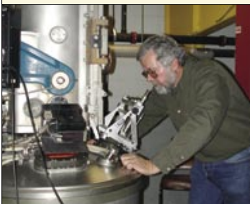
Lance Falkenstein monitors a growth chamber, which operates at over 2000 deg. F
