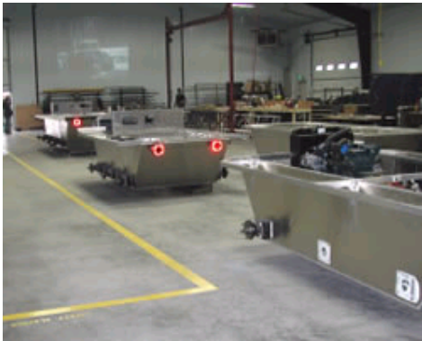
Land Tamer all-aluminum platforms in stages of assembly (SWIP) at May 28 open house; containment walls will be completed after flow decisions finalized.
