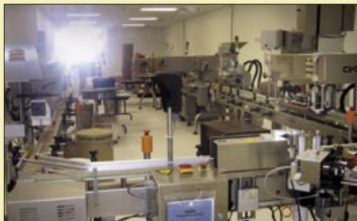
Automated capsule and tablet filling line increase capacity.
