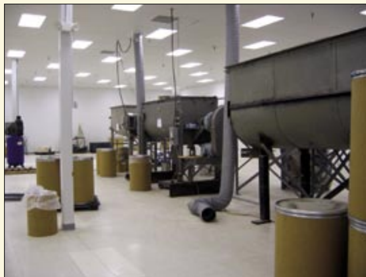
Cone, paddle and ribbon blenders are capable of mixing from 300 to 10,000 pounds of ingredients at one time.
