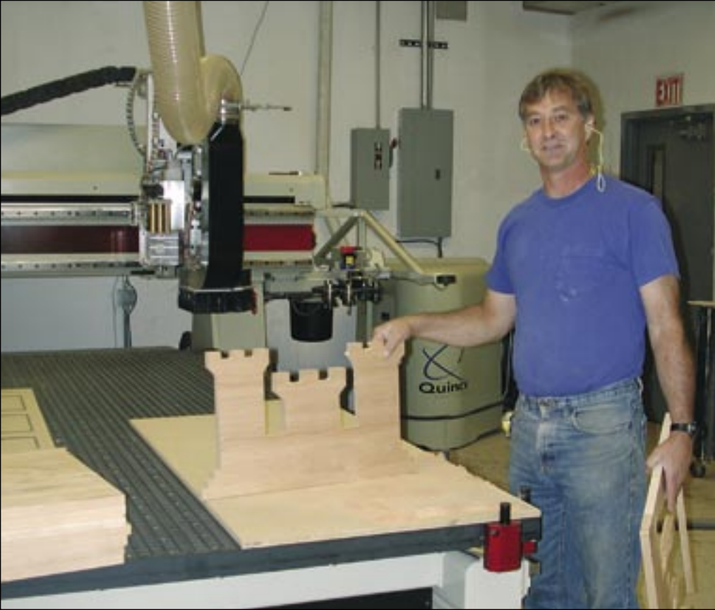
Gerald poses with the CNC router that uses an Autocad program that accepts and converts the code from many graphics programs. It reduces his drawing time on projects and provides greater convenience for customers. This drawing of a castle was received in Corel Draw.
