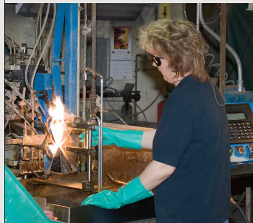
Sherry brazing handles together on the automated brazing machine.
