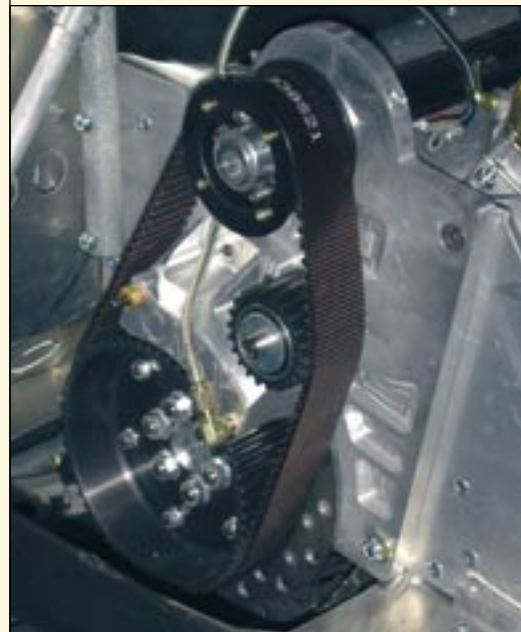
Crazy Mountain Motorsports was the first to offer a belt drive system (CMXDS) as standard equipment as well as offer it in kit form for upgrading older heavy chain case drive systems on other machines.
