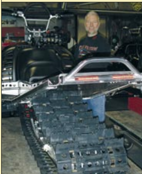
Well protected in the bumper, the light weight LED tail light array fits CMX design and look as new sled takes shape.
