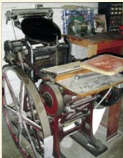
1895 era press was converted for electricity; still has uses today.
